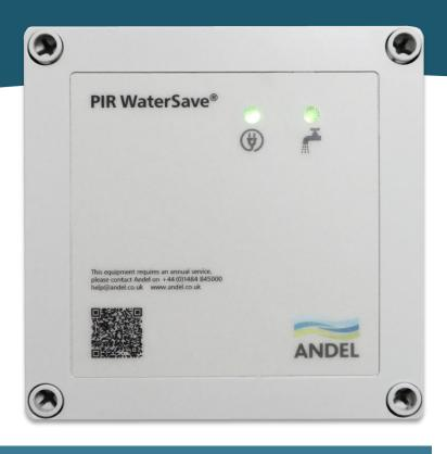
The PIR WaterSave® system comprises of a wall-mounted control panel and a 360° PIR (Passive Infra-red) motion sensor which together control low-energy, motorised isolation valves, switching the water supply on and off as required, through the detection of movement in the monitored area.
